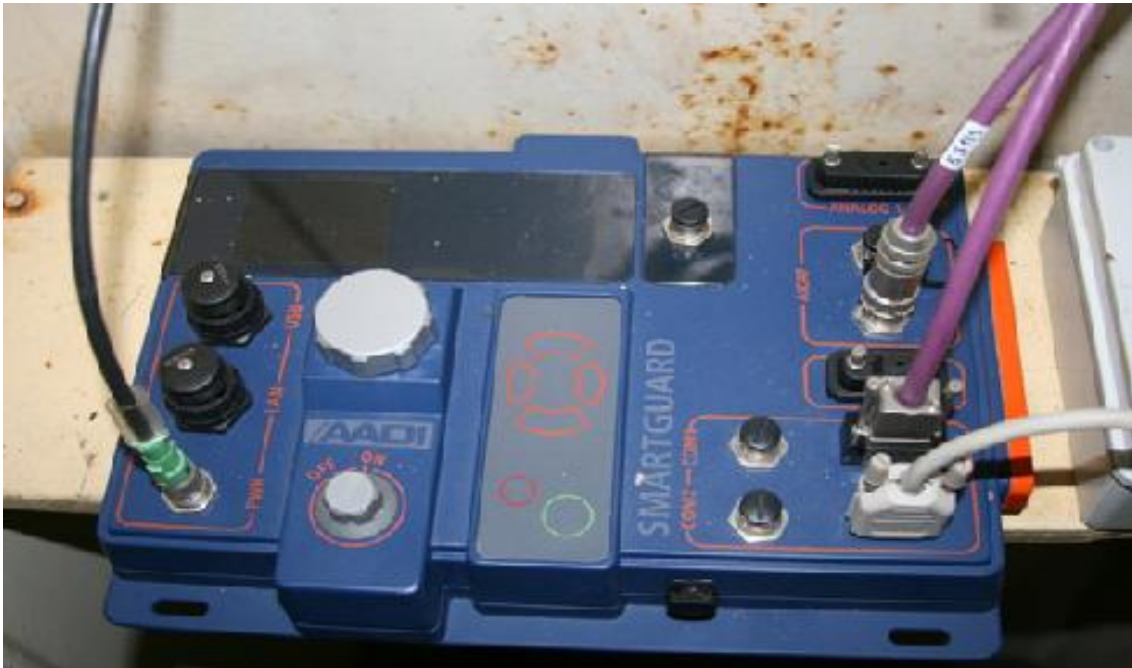
Figure 11 Datalogger SmartGuard from Aanderaa Data Instruments on M/S ROMANTIKA, that collected all data from different sensors installed in FerryBox chamber. For data logging and transmission, additional sensors can be connected to the logger. [22]
