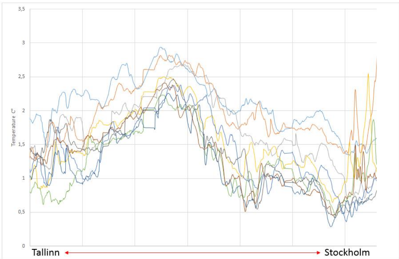
Figure 26 Seawater temperature as measured along ship track on Tallinn-Stockholm and Stockholm-Tallinn routes during 9 trips (5.02.2017-14.02.2017).
