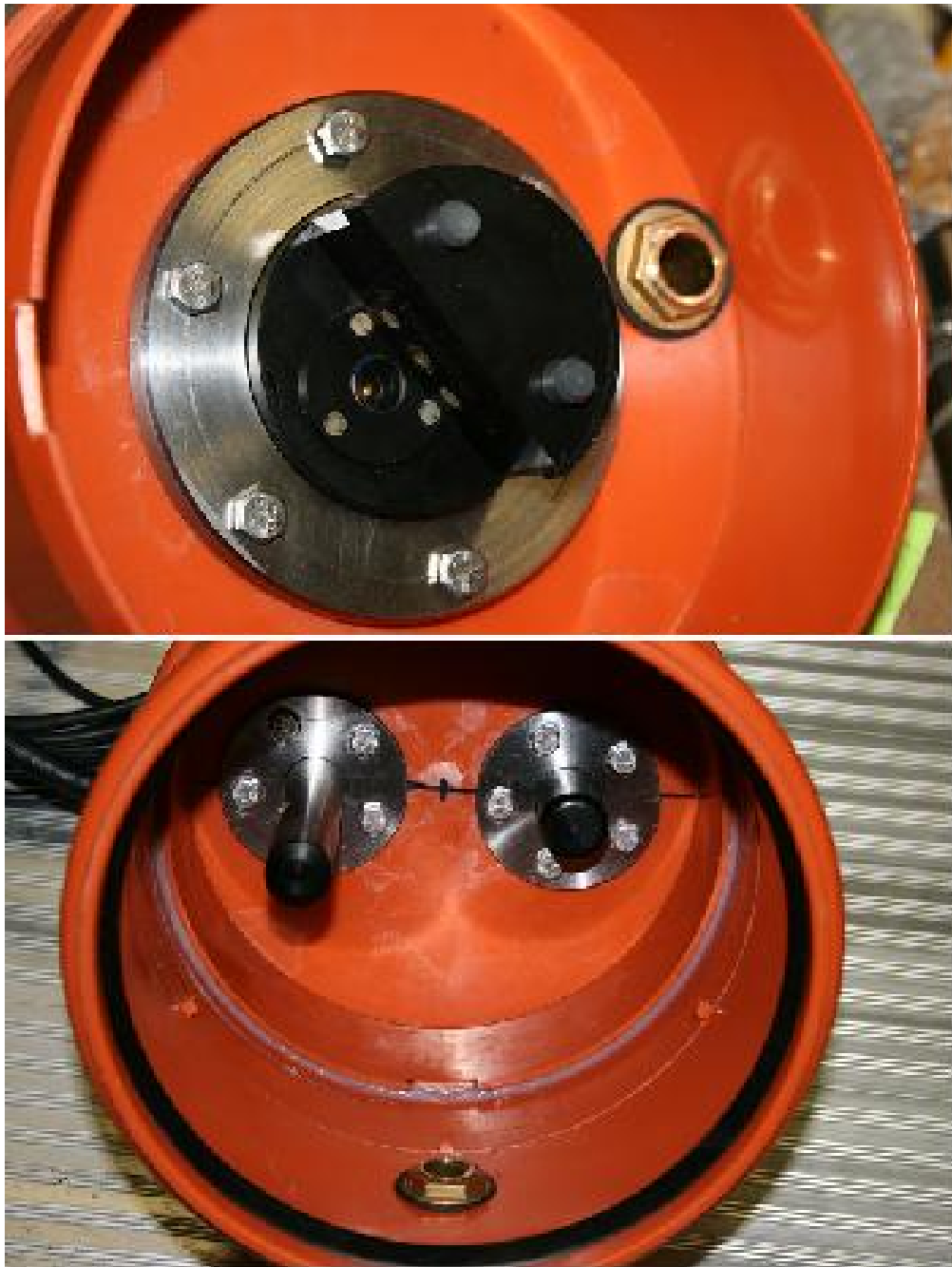
Figure 13 Sensors on FerryBox system aboard M/S BALTIC QUEEN. In the upper picture UviLux sensor for PAH detection and on the lower for conductivity and temperature, 36 Xi W by KELLER (left) and Seapoint Turbidity Meter (right).
